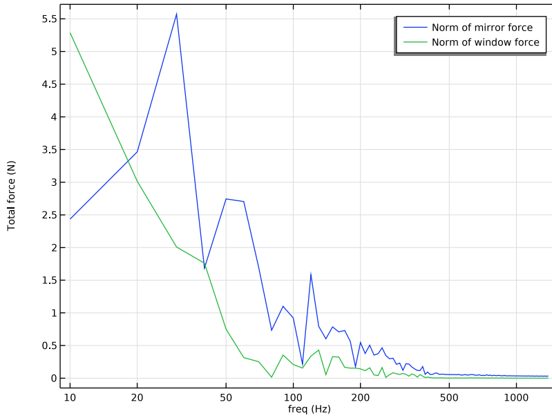
Figure 2: Integrated total force magnitude on the window and side mirror as a function of frequency.
