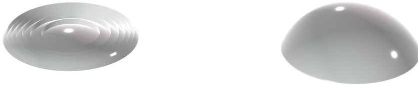
Figure 1: Comparison of a Fresnel lens (left) with a plano-convex lens (right) with similar focal length. The Fresnel lens is much thinner and lighter.
