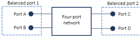
Figure 2: Balanced port configuration of a four port network in the mixed-mode S-parameter feature.
