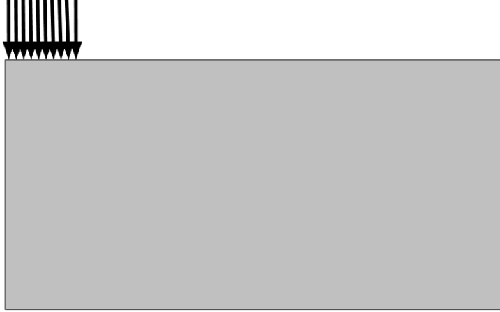
Figure 2: Model geometry and indentation load for the second benchmark test. The simulation is performed on the symmetry plane in 2D.
