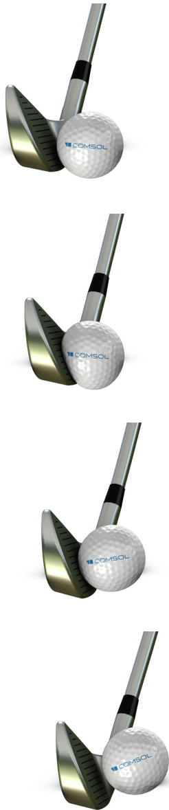
Figure 2: Snapshots of the club and golf ball during the simulation. From top to bottom, the timings are 0 ms, 0.15 ms, 0.30 ms, and 0.45 ms.
