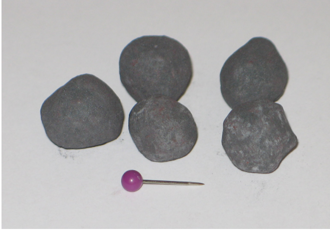
Figure 1: Hematite pellets after drying and oxidation (end product).
