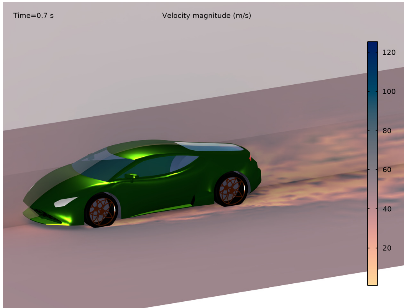
Figure 8: Slice plots of the velocity magnitude from the LES solution at t = 0.7 s.
