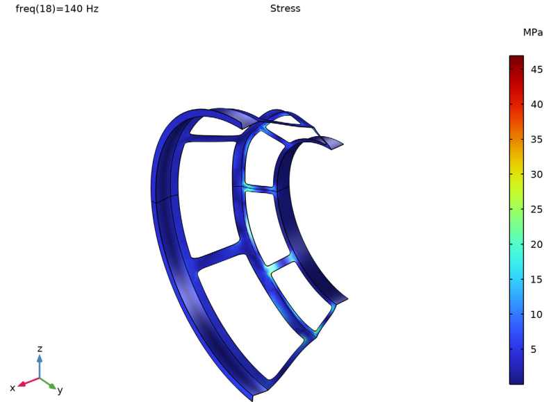
Figure 9: Stress distribution at 140 Hz on the basket.
