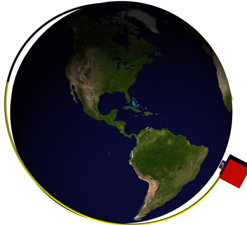
Figure 6: Orbit of a satellite around the Earth. The track color indicates whether the satellite is in eclipse or not. The spacecraft surface color represents the magnitude of the incident solar irradiation.
