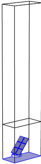
Figure 4: Computational box used in the fluid-flow simulation.
