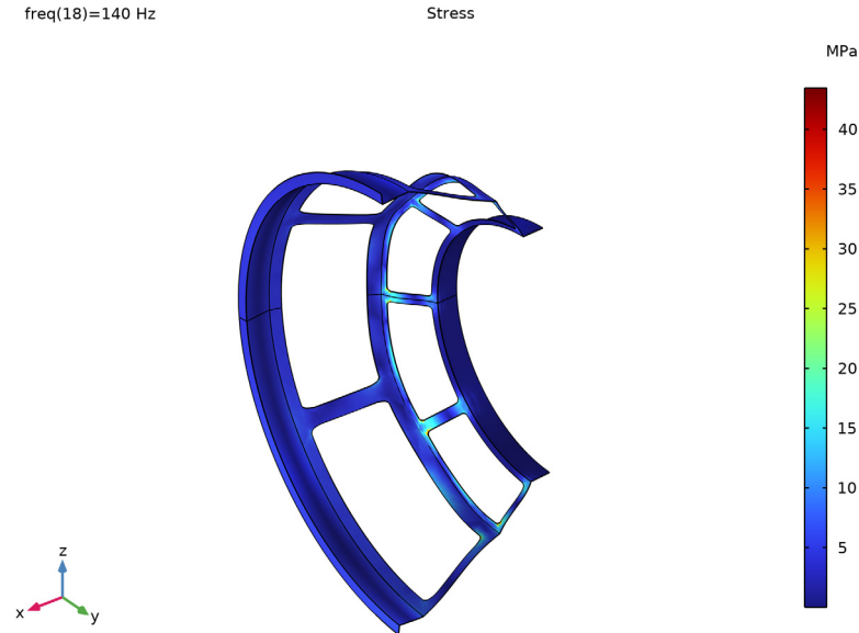
Figure 9: Stress distribution at 140 Hz on the basket.
