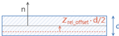
Figure 5-7: Meshed boundary indicated in red. The vector \mathbf{n} indicates the positive orientation of the boundary normal.
