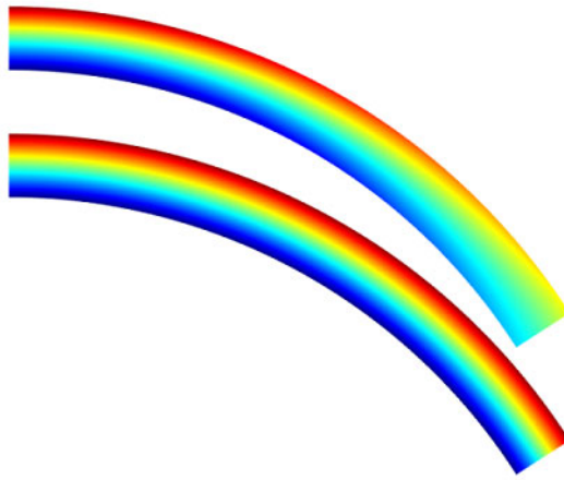
Figure 2-15: xx -components of the Cauchy stress tensor (top) and the second Piola–Kirchhoff stress tensor for an initially straight beam.
