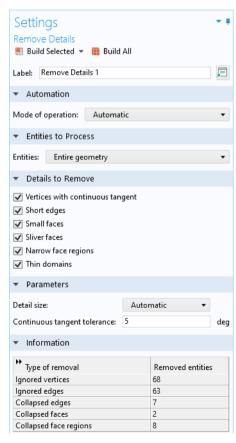
be needed. The fastest way to determine if this is the case is to build the mesh and check if the mesh generator displays any Information about small entities.
