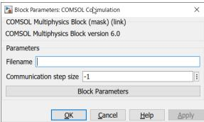
In the Filename field enter the cosimulation filename. If you do not enter the full path for the cosimulation file, the COMSOL Cosimulation block searches in the following locations in the order they are listed below:
