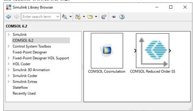
The COMSOL Cosimulation block can be used as any Simulink block; for instance, to add it to the Simulink diagram, drag and drop the block.
