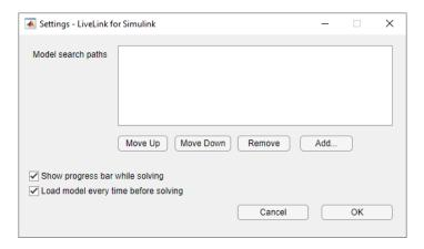
Use the **Add** and **Remove** buttons to update the MATLAB search path with the path of the model to run in cosimulation with Simulink.
