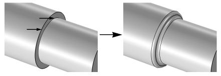
To open the Tools window for Delete Fillets, from the Geometry toolbar, Defeaturing and Repair ( 1 menu, select Delete Fillets ( 1 ). You can also right-click the Geometry node and select the same option from the context menu.
