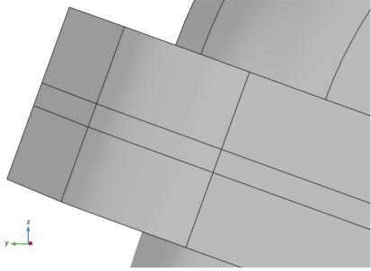
The thin domain is automatically detected and removed by Remove Details.
