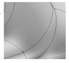
The sequence of virtual operations generated by Remove Details includes several other Ignore Edges and Ignore Vertices operations to remove slivers
