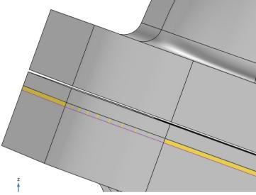
It seems that in addition to the overlap there is also a gap between the gasket and the manifold. This is also evident since the interference detection tool did not find any touching boundaries. Try to increase the tolerance for the Detect Interferences tool in order to detect and get a measurement of the gap.
