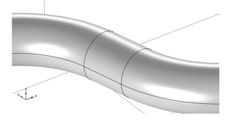
The Cap Faces operation, which you will use to create a domain inside the manifold, needs an input in form of the bounding edges of the empty volume that should be turned into a solid. For this exhaust manifold these are the edges highlighted in the figure below.
