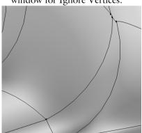
The sequence of virtual operations generated by Remove Details includes several other Ignore Edges and Ignore Vertices operations to remove slivers with increasing face width. In the following take a closer look at the *Collapse Face Regions* operation, that is added to the sequence to detect and remove narrow face regions.
