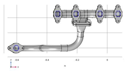
You could select these edges directly in the Cap Faces operation, however a more efficient way, which only requires the selection of one segment from each edge loop, is to use an Explicit Selection where you have the option to automatically include continuous edges in the selection.
