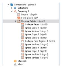
geometry may only need one pass, but with a more complex geometry, like this wheel rim, the Remove Details operation goes through three passes and a cleanup pass at the end. Take a closer look at some of the virtual operations in the sequence.
