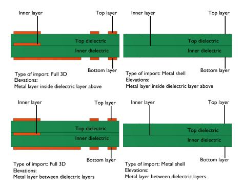
The Full 3D option imports all copper layers with a thickness according to the Layers to import table. The layer elevations are determined according to Elevations, see in the next section Controlling The Layer Stackup. With the Metal shell option copper layers are imported as embedded boundaries between dielectric regions. As illustrated in the figure above, switching to Metal shell changes the elevation of dielectric layers when Elevations is set to Metal layer between dielectric layers.
