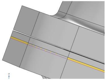
It seems that in addition to the overlap there is also a gap between the gasket and the manifold. This is also evident since the interference detection tool did not find any touching boundaries. Try to increase the tolerance for the Detect Interferences tool in order to detect and get a measurement of the gap.
