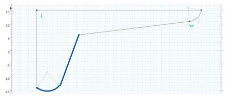
7 Next add constraints to position the centers of the circular arcs to lie on the two straight edges. First select the horizontal edge and the center of the circular arc
