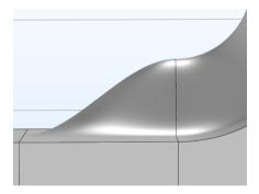
The overall result is better compared to the Parallel loft direction, since the constraint on the tangent influences the entire surface, even though it is applied only at the vertices.
