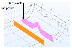
While in this case the input consists of a start and an end profile, it is possible to define additional profiles in the Profiles section.
