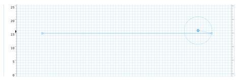
**6** Move the mouse to form the arc, then click to place a vertex where the arc ends.
