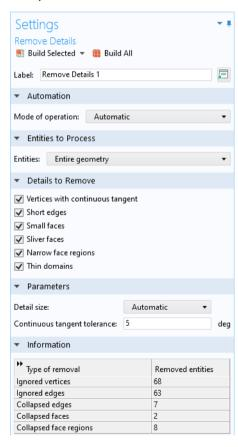
determine if this is the case is to build the mesh and check if the mesh generator displays any Information about small entities.
