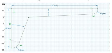
The applied constraints and dimensions are now sufficient to define the shape, but the two translational rigid body degrees of freedom are not yet constrained.
