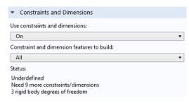
underdefined, and it needs 9 more constraints or dimensions. The rigid body translational and rotational degrees of freedom are not yet locked, meaning that the entire sketch can be moved around freely as a rigid body. To lock the rotational degree of freedom you can for example apply the *Vertical* or *Horizontal* constraints to an edge.
