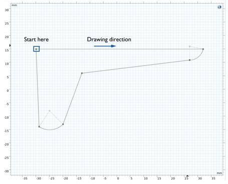
**3** Move the pointer to the right, and at the end of the first edge where the circular arc starts click once to place a vertex.
