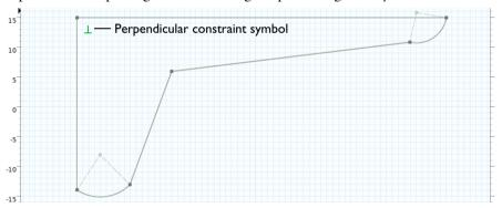
Note that in the Model Builder, the Perpendicular 1 node has been added under the geometry sequence. Similar to all other geometry features, you can select the node to change its settings. 4 Select the circular arc and straight edge highlighted below.
