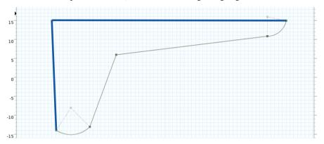
The perpendicular constraint is suggested, and its symbol appears under the pointer.
