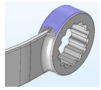
5 In the Settings window for Boundary Load, under Force, select Total force as the Load type and enter -F in the text field for the z component.
