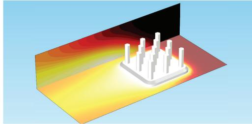
It's a little easier to see what's going on now; the contour layers show the evolution of the temperature gradient on the back wall, which is at its hottest right next to the heat sink. The contours are very smooth already (try refining your mesh to get the smoothest results), but let's add the lines back in so that we can get a really clear idea of the temperature gradient.
