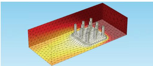
Now we can see that the mesh is finest around the heat sink and pillars, and less refined on the air domain walls. If we were to disable the temperature surface, we would see only the wireframe lines. Like other plot types, wireframe surfaces can be plotted on different data sets, and their coloring and style settings may be adjusted to your liking.
