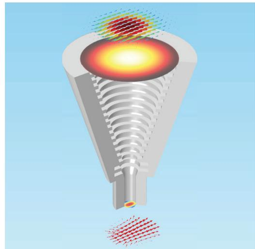
Create a new solution under the Results node, Study 1/Solution 1 (5). Add a selection that includes domains 3, 4, and 6 (the horn, feed, and aperture). Then right-click Data Sets and choose *Revolution 2D*. Choose Study 1/Solution 1 (5) as the data set and use a start angle of -90 degrees and a revolution angle of 225 degrees.
