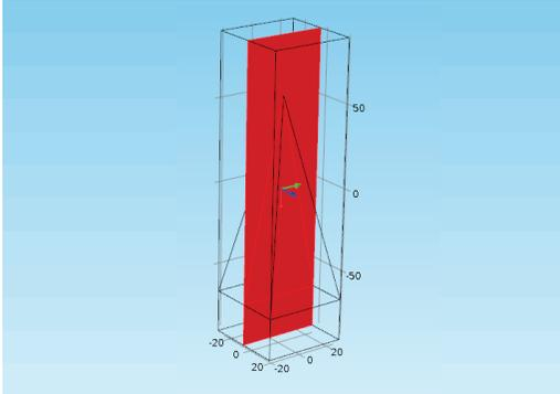
Go back to the Surface node in 2D Plot Group 3, make sure that the data set is set to *Cut Plane 1*, and click Plot. Now we have results:
