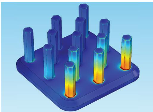
This new plot shows something that the old surface didn't: the energy transfer on the pillars of the heat sink nearest to the inlet (rotated toward the front in the previous image) is happening at a much higher rate than the transfer near the outlet. In fact, there are some pillars that don't seem to have much heat transferring at all; it's possible that these could be removed from the design to save money and material.
