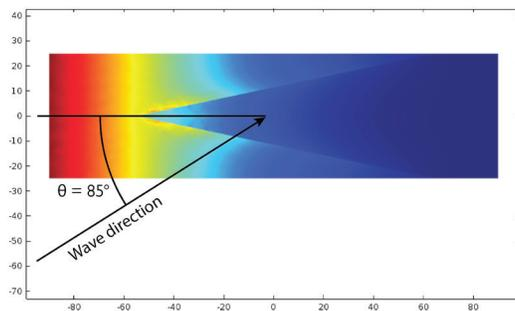
This surface plot is based on a chosen elevation angle of  $\theta = 1.48353$  (85 degrees), which is the largest elevation angle (that is, the largest angle of incidence of the wave) that applies to this pyramidal unit cell.
