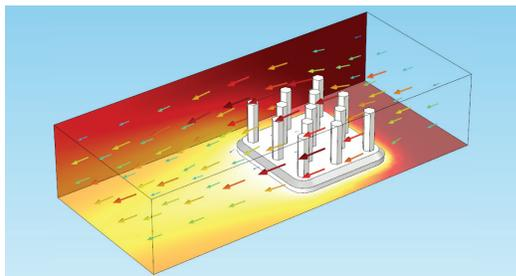
Now the arrow plot shows the velocity of the airflow as it changes. The *Color legend* check box under the Coloring and Style tab allows you to see a reference for the fastest and slowest flow regions (with red being the fastest, blue the slowest).
