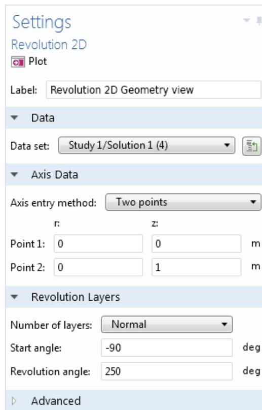
The Axis Data and Revolution Layers sections contain information that determines how far the revolution is and around which axis.
