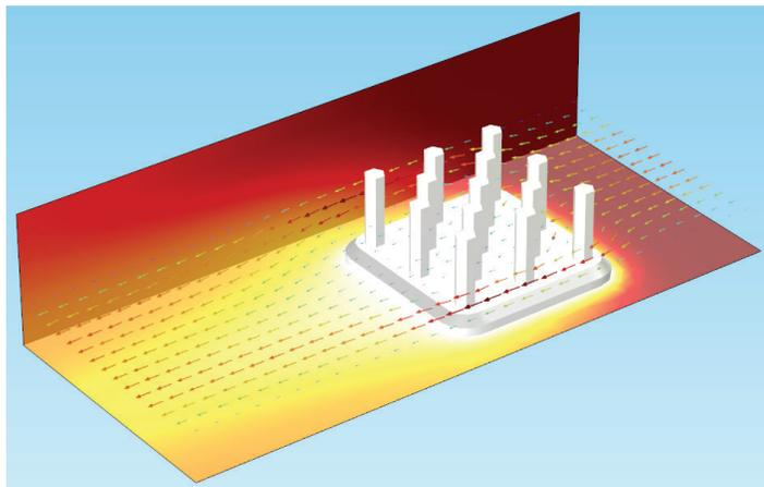
Your initial arrow plot won't look like the one above, though; to create the above image, you would need to add more arrows, and would have to scale them down so that the geometry underneath is visible.
