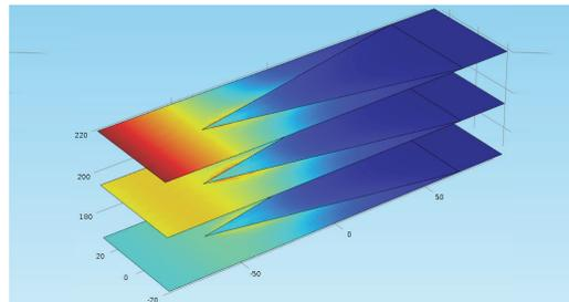
We've made a parametric extrusion. The different slices show the electric field on the pyramidal unit cell for the selected values of  $\theta$ .
