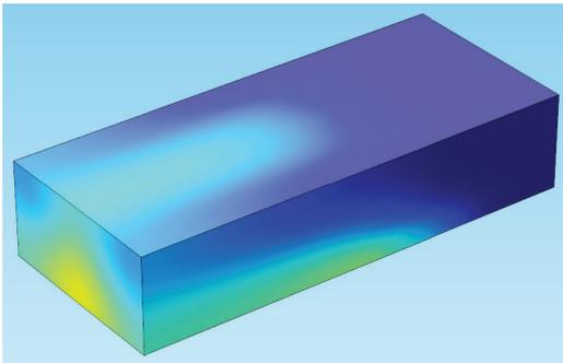
In the Surface settings window, we can change this under the Coloring and Style tab. Using the drop-down list, change the color table from Rainbow to ThermalLight.
