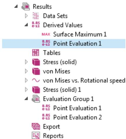
In the geometry shown in the Graphics window, a set of points will appear on the pulley cross-section. These are points that are drawn in the model geometry. One or more of them must be selected for the point evaluation (we can't choose a point just anywhere, as in the case of a cut point). These points can also be added to an *Evaluation Group*, which allows multiple *Point Evaluation* nodes to be computed simultaneously.
