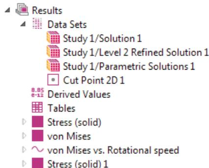
Three solutions have already been created. They are different result sets from the same study; Study 1/Level 2 Refined Solution 1 includes a step in the study that refines the mesh in certain areas of the model where greater accuracy is needed, while Study 1/Parametric Solutions 1 includes results from the parametric sweep performed in the study.
