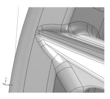
recommended to use a small tolerance together with the repair operation. If preserving the surface curvature is important for the analysis, virtual geometry operations, which work by hiding geometry features from the mesher, are available as an alternative. How you can do this is described further ahead, in the tutorial *Removing Small Geometric Entities Using Remove Details*.
