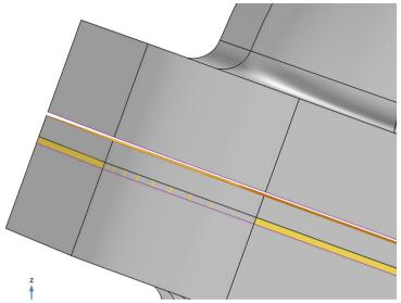
This time the gap is detected. The gap distance is displayed in the Interfering faces list, and it is 0.4 mm.
