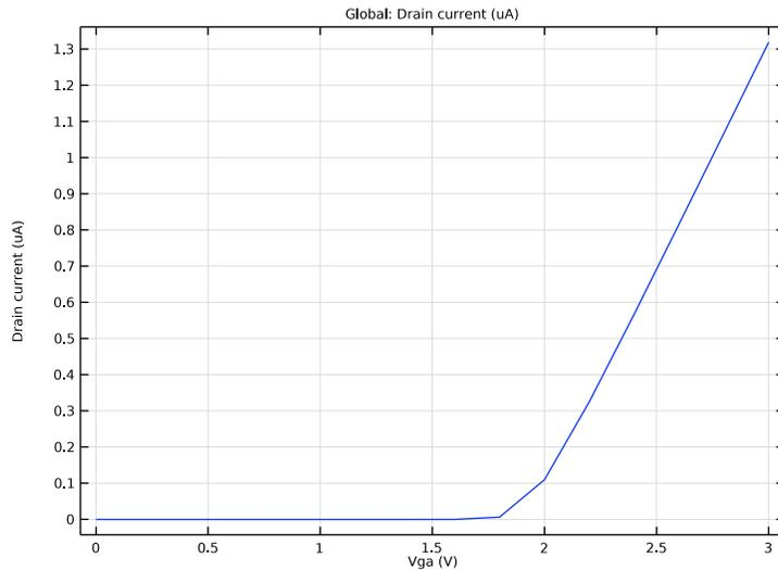
The figure indeed shows the same  $I_d$ - $V_g$  behavior as one would observe in a typical MOSFET.
