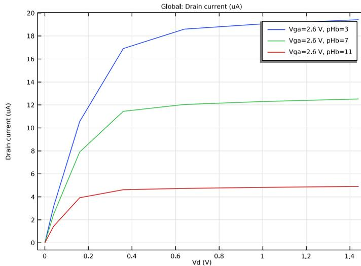
Note that the  $I_d$ - $V_d$  curve of the ISFET is modulated by the pH value of the bulk electrolyte, in exact analogy to how the  $I_d$ - $V_d$  curve of a MOSFET is modulated by the gate voltage. In other words, the effective gate voltage seen by the ISFET is modulated by the pH value of the bulk electrolyte. This provides the basic sensing mechanism for measuring the pH value.
