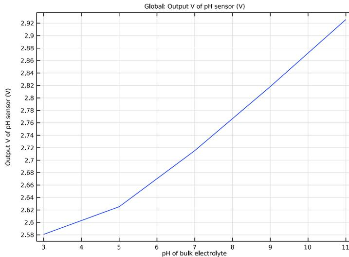
Figure 4: Sensitivity curve for the ISFET pH sensor.
