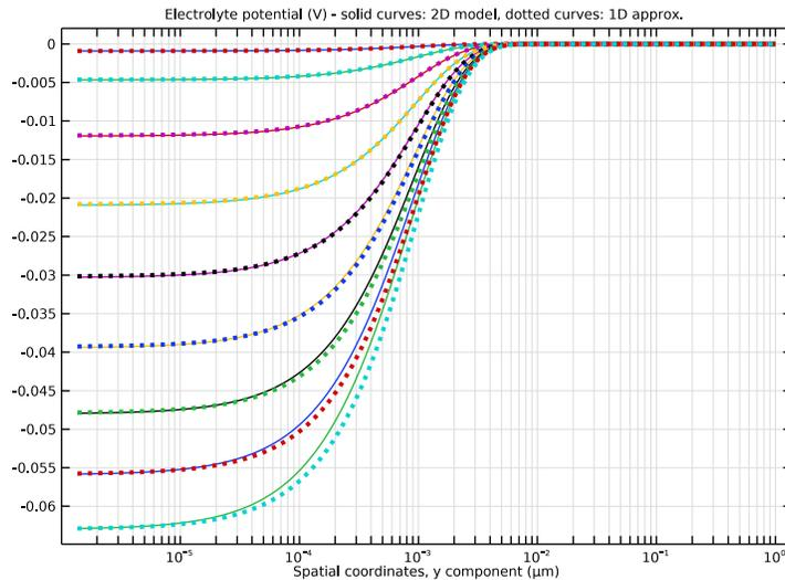
The 1D approximation reproduces the general trend of the electrolyte potential along the centerline of the electrolyte domain, as one would expect.
