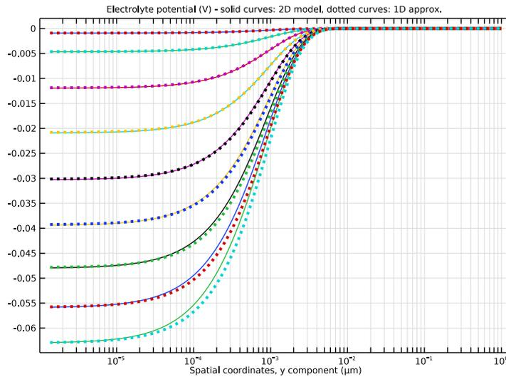
Figure 1: Electrolyte potential along the centerline of the electrolyte domain. (It does not extrapolate to the dielectric surface potential at  $y=0$  because the voltage drop across the Stern layer is not explicitly modeled in the electrolyte domain. See [Model Definition](#) for details.)
