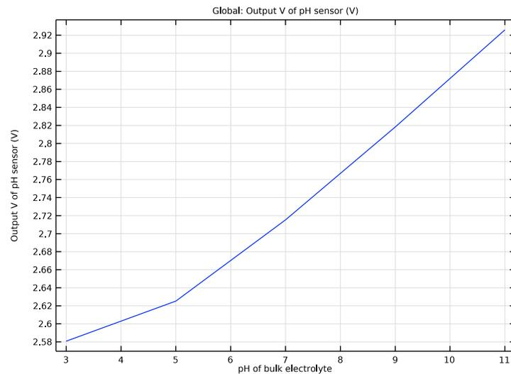
The sensitivity of the ISFET is given by the slope of the curve. The result is consistent with the one reported in the reference paper.
