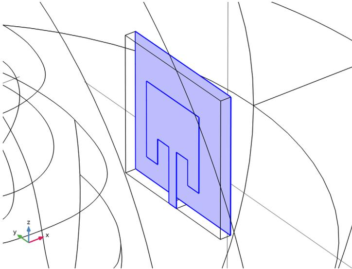
The metal parts of the antenna substrate are defined as perfect electric conductors, assuming that the conductivity of copper is high enough to have negligible loss.
