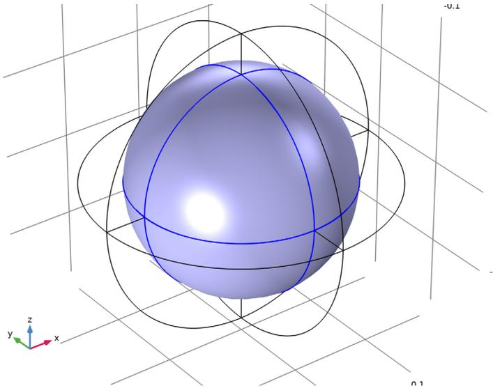
The **Far-Field Domain** feature defines a wave number for use by its subfeature - the **Far-Field Calculation** feature.
