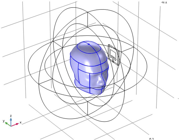
The specific absorption rate feature defines the SAR postprocessing variable. It is calculated from the electromagnetic dissipation density and the specified density for the human head.
