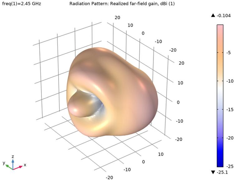
The far-field radiation pattern of the microstrip patch antenna is distorted due to the reflection from the human head.
