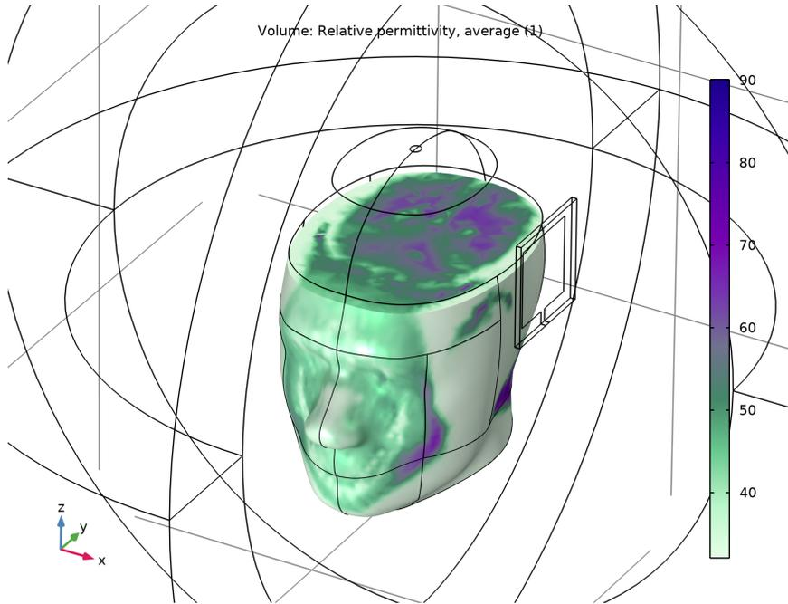
*Figure 1: This plot shows how the average relative permittivity varies inside the head. The permittivity is calculated from the imported MRI image data.*
