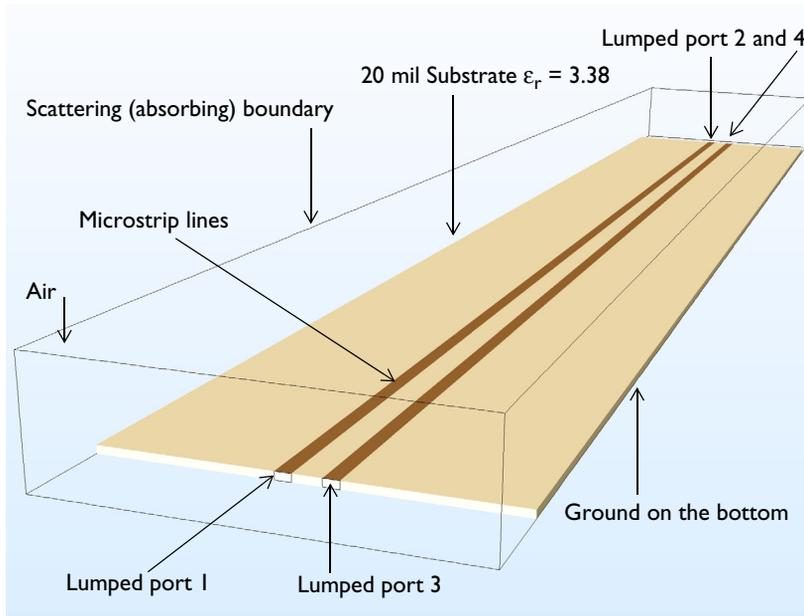
*Figure 1: A microstrip line crosstalk model is composed of 20 mil microwave substrate with a ground plane and two adjacent microstrip lines 1.8 mm apart.*
