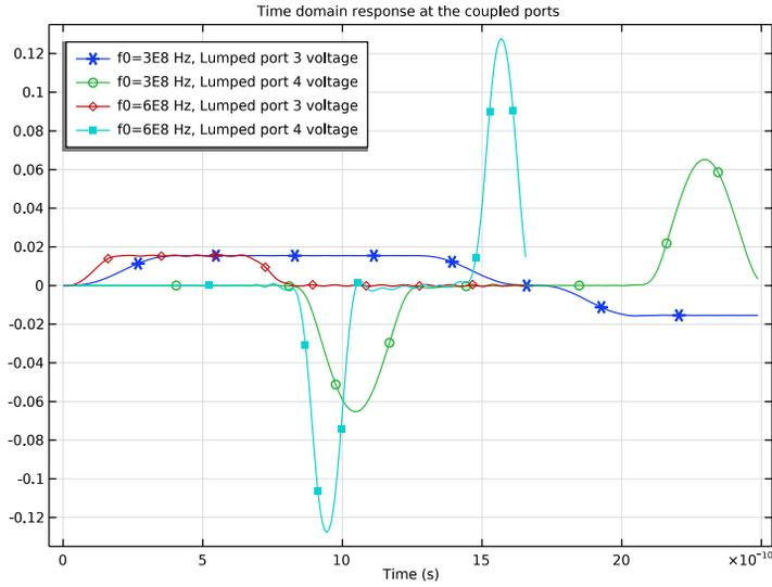
Figure 4: Voltage for the coupled signals at lumped ports 3 and 4. They are near-end crosstalk (NEXT) and far-end crosstalk (FEXT), respectively. The voltage of a coupled signal increases at a higher data rate.
