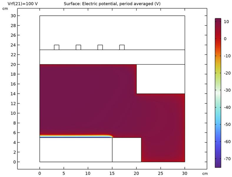
Figure 3: Period averaged electric potential for 250 W of coil power and  $V_{rf} = 100$  V.
