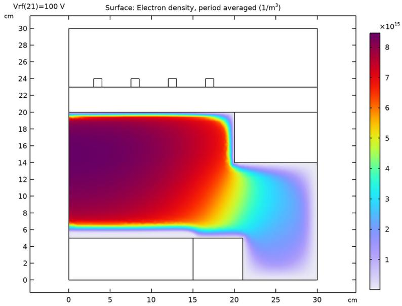
Figure 1: Period averaged electron density for 250 W of coil power and  $V_{rf} = 100$  V.
