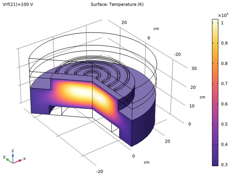
Figure 6: Gas temperature for 250 W of coil power and  $V_{rf} = 100$  V.
