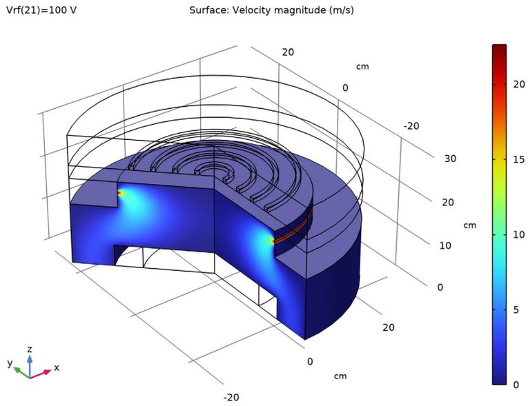
Figure 5: Magnitude of the fluid velocity for 250 W of coil power and  $V_{rf} = 100$  V.
