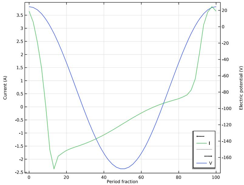
Figure 4: Current and voltage at the biased electrode for 250 W of coil power and  $V_{if} = 100$  V.
