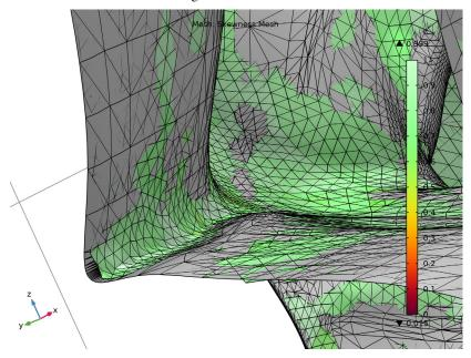
It is clear that the mesh of the generated geometry (green) does not follow the source mesh (gray) closely in the region of the 90 degree corner. In regions with lesser curvature the green and gray mesh elements are more intermixed. This indicates better conformance of the generated mesh to the source mesh in those regions.
