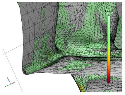
The mesh of the generated geometry (green) now follows the source mesh (gray) much closer. This is the effect of the smaller Relative simplification factor, which allows for less deviation from the source mesh when the surface is generated during import.
