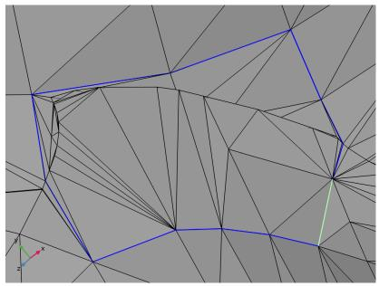
3 In the Settings window for Create Edges, click 📳 Build Selected to generate the edges and partition the boundary.
