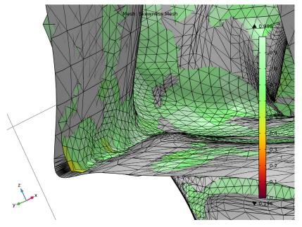
Looking at the same corner region, the mesh of the generated geometry (green) shows a more rough representation of the source mesh (grey). This is expected as increasing the Relative simplification factor allows for a larger deviation from the source mesh when the surfaces of the geometry are generated during the import.
