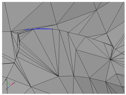
The two edges are located at the fold in the mesh. Open the **Selection List** again, make sure **Select Boundaries** is selected, and notice that Boundaries 2 and 3 are in the same location as the short edges on the generated geometry. These are isolated boundaries on the outside of the surface mesh and are attached to the mesh only through a single edge.
