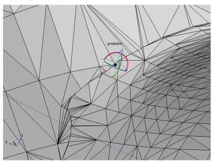
These intersecting elements can be fixed with a mesh **Union** operation with an absolute repair tolerance of 0.1 mm. However, this is not needed here as the simplification done when creating a geometry of the mesh takes care of this.
