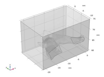
The resulting object now contains two domains, inside and outside the imported geometry. Using a transparent view can help to see the parts inside the block. Continue with finalizing the geometry and creating a mesh.
