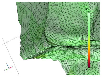
The generated geometry face is smooth and has a **Geometric Shape Order** corresponding to the discretization of the physics in the model. In practice, this means that the Geometric Shape Order is most often quadratic, unless solving a CFD problem, where linear discretization is used. To plot the curved elements on the boundary, change the corresponding setting on the dataset.
