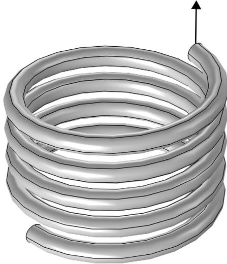
*Figure 1: A 4.5-turn steel spring is fixed at one end, and has a load applied at the other. The load is a variable which is solved for to achieve a total displacement.*
