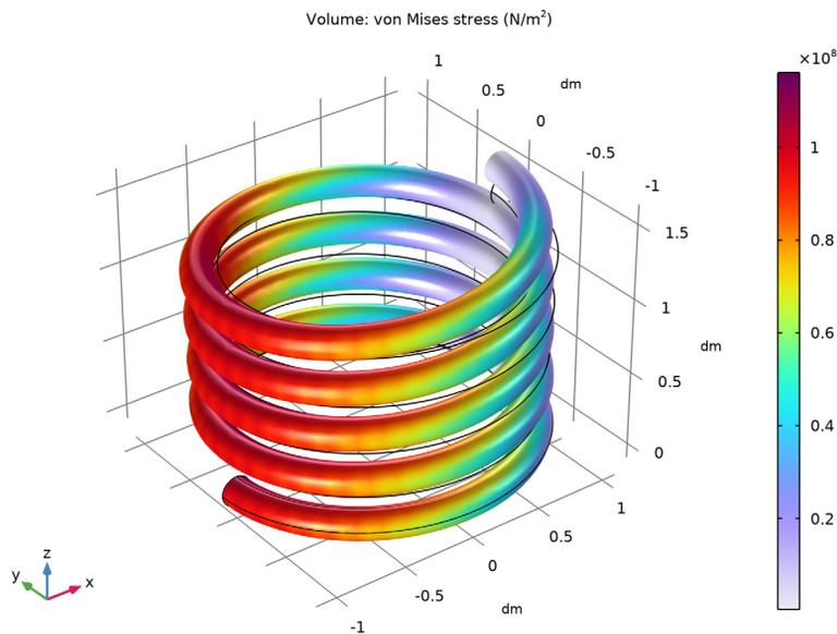
Figure 2: The deformed shape of the spring.
