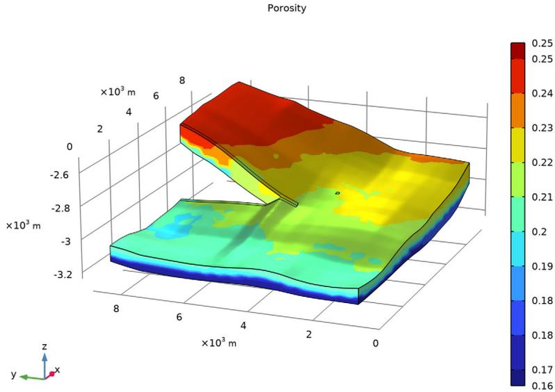
Figure 1: The porosity in the of the part of the Johansen formation that is used for the simulation.
