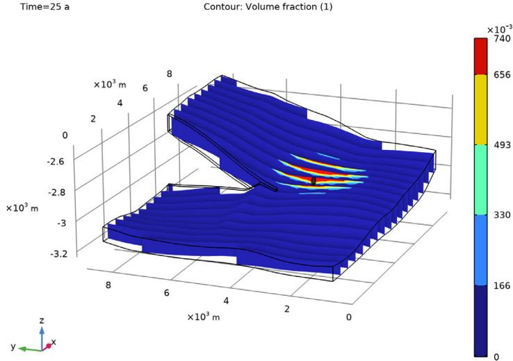
Figure 3: The CO<sub>2</sub> saturation after 25 years of injection.
