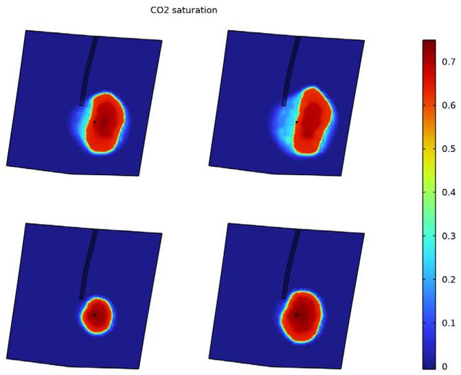
Figure 4: Top view of the formation showing the CO<sub>2</sub> saturation after 12.5 years (bottom left), after 25 years (bottom right), after 37.5 years (top left), and after 50 years (top right).
