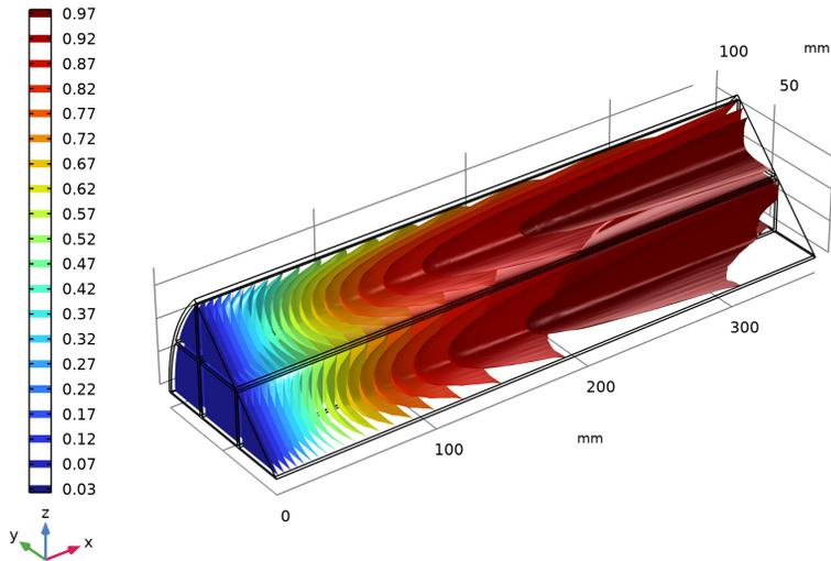
Figure 3: Isosurfaces showing the conversion of NO in the reactor. Fluid flow from left to right.
