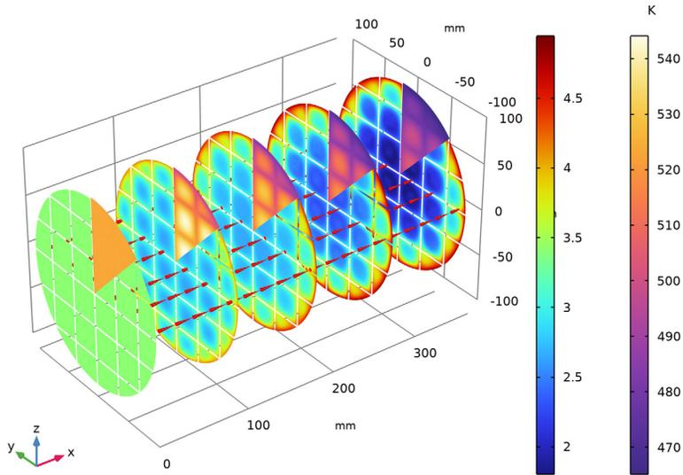
Figure 5: Selectivity (leftmost color legend) and temperature in slices throughout the monolith reactor. Fluid flow from left to right.
