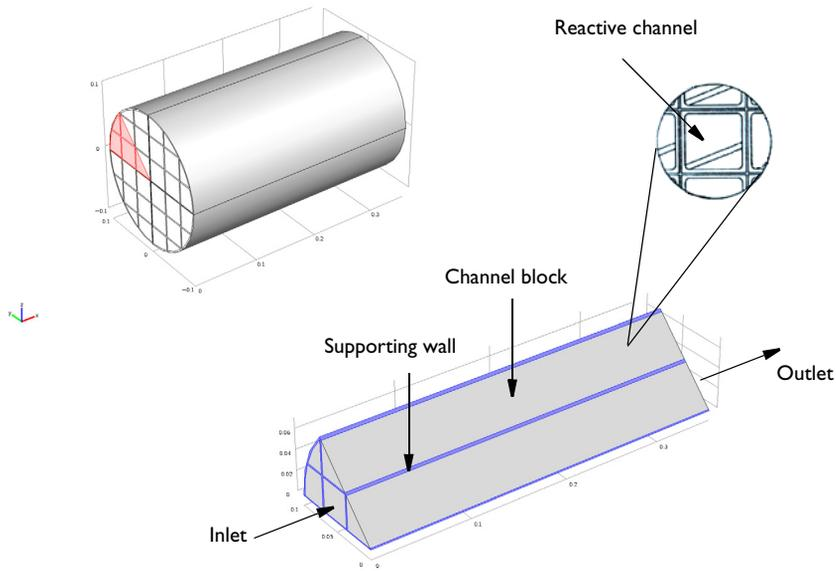
*Figure 2: NO reduction chemistry takes place in the channel blocks. Supporting walls hold together the full reactor geometry. Symmetry reduces the modeling domain to one eighth of the full reactor geometry.*
