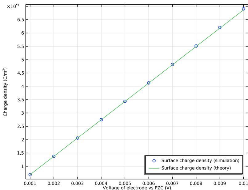
Figure 3: Surface charge density as a function of applied potential difference between the electrode and bulk solution, comparing simulation results with analytical theory derived in the limit of low applied potential.
