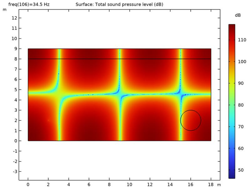
*Figure 1: The initial design has a pressure node at the edge of the objective domain.*
