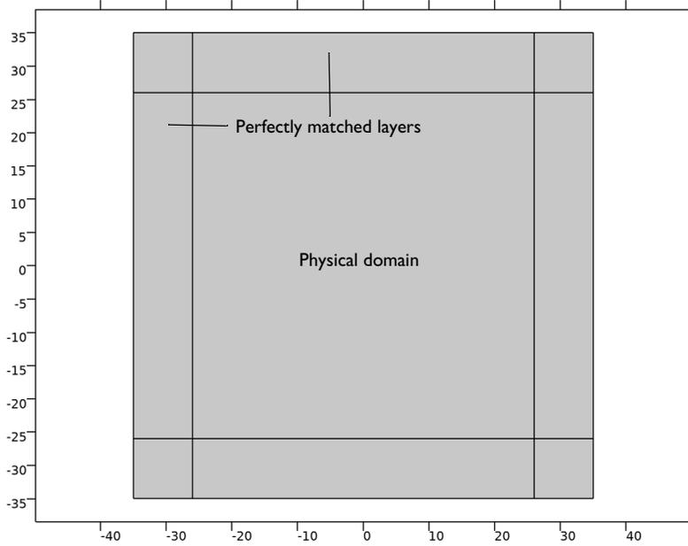
Figure 1: Geometry: physical domain and perfectly matched layers.
