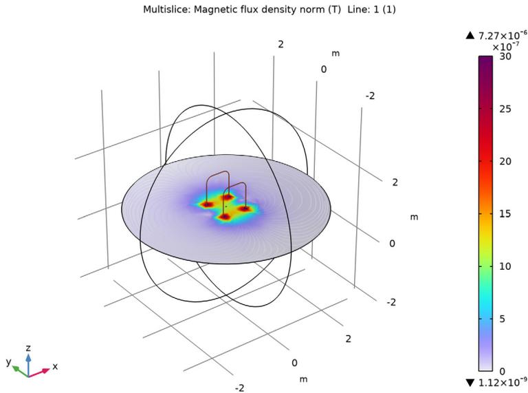
As a final step, evaluate the mutual inductance by integrating the magnetic vector potential along the transponder coil; first, analyze the verification of the intended transponder coil direction, then perform the integral.
