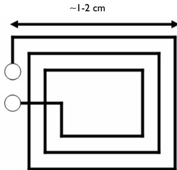
and a common type of reader antenna is a larger dual coil:
