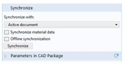
By this action you transfer the geometry of the pacemaker electrode from Solid Edge to COMSOL.
