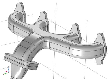
The holes are now deleted, and, similarly to the previous defeaturing operation, a Delete Holes 1 (dho1) node is inserted into the geometry sequence just above the Union 1 (uni1) node.
