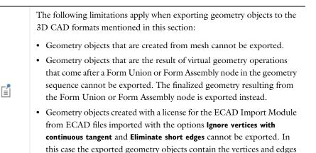
COMSOL objects are automatically converted to CAD objects before saving the file.
