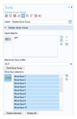
deleted you can edit the settings for the operation to set a tolerance that is just slightly larger than the width of the face.
