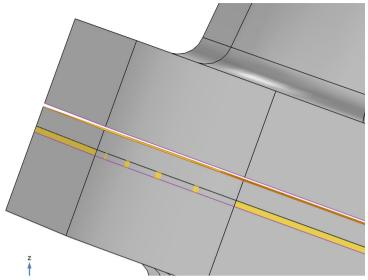
This time the gap is detected. The gap distance is displayed in the Interfering faces list, and it is 0.4 mm.
