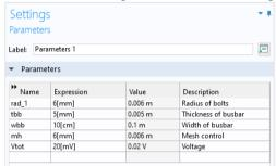
To keep the existing parameters in a model unmodified by the import, you can clear the Overwrite check box in the Excel Load dialog box before the import. In this case, imported parameters will be appended to the table and you will need to resolve any conflicts between similar parameter names yourself.
