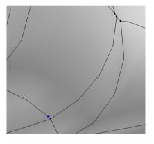
The sequence of virtual operations generated by Remove Details includes several other Ignore Edges and Ignore Vertices operations to remove slivers
