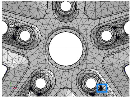
The areas of dense mesh close to each bolt hole are due to slivers and small faces.
