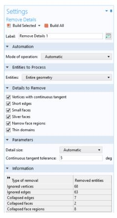
be needed. The fastest way to determine if this is the case is to build the mesh and check if the mesh generator displays any Information about small entities.
