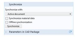
By this action you transfer the geometry of the pacemaker electrode from PTC Creo Parametric to COMSOL.
