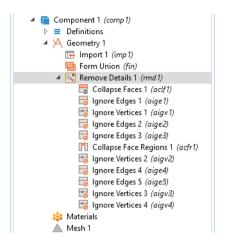
geometry may only need one pass, but with a more complex geometry, like this wheel rim, the Remove Details operation goes through three passes and a cleanup pass at the end. Take a closer look at some of the virtual operations in the sequence.
