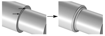
To open the Tools window for Delete Fillets, from the Geometry toolbar, Defeaturing and Repair ( ) menu, select Delete Fillets ( ). You can also right-click the Geometry node and select the same option from the context menu.
