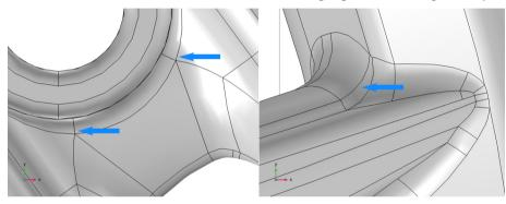
The small faces and slivers are no longer present in the geometry. According to the Information section in the Settings window for Repair, 60 short edges and 20 sliver faces were removed.
