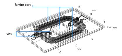
4 Note the additional objects and named selections that appear in the Selection List window. The import extrudes drill layers separately for each dielectric layer, and names these by combining the name of the drill and dielectric layers. For example the ferrite core, generated from the THROUGH.HOLES layer is extruded into two separate objects: THROUGH\_HOLES\_INNER\_LAYER\_DIEL and THROUGH HOLES TOP LAYER DIEL.
