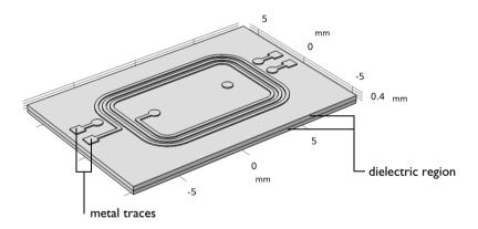
The import can be configured to use one of 3 methods to generate 3D solid objects from the 2D layouts and group these together:
