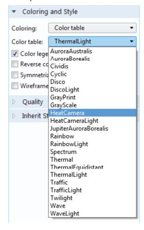
Other settings in the Coloring and Style section allow you to control whether the color legend is visible in the Graphics window and how the color range is chosen. For instance, selecting the Reverse color table check box will reverse the color order in the gradient while the Symmetrize color range check box will center the color range at a results value of 0.
