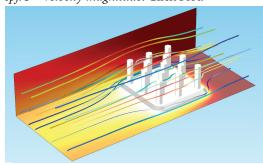
You can also position streamlines according to a plane or line. Set the Positioning field to Start point controlled and use the dropdown menu for Along curve or surface to select the desired line or plane.
