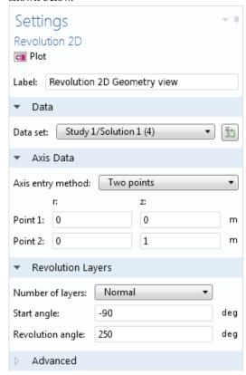
The Axis Data and Revolution Layers sections contain information that determines how far the revolution is and around which axis.
