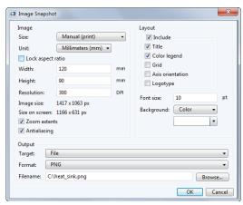
Setting the size to *Current* exports the exact image shown on the screen. There are also two options for *Manual*, which allow you to control the dimensions of the image. With these options, you can export an image with resolution intended for print or web viewing.
