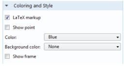
change the coloring and style settings to change the text and background color or include a frame around the note.
