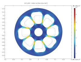
The solution to this model is found using a kinetostatic analysis, where the pulley is "frozen" at a moment in time and the center is assumed fixed. We can examine the stress distribution and deformation for different rotational speeds (the variable *n* represents the rpm).
