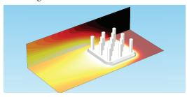
It's a little easier to see what's going on now; the contour layers show the evolution of the temperature gradient on the back wall, which is at its hottest right next to the heat sink. The contours are very smooth already (try refining your mesh to get the smoothest results), but let's add the lines back in so that we can get a really clear idea of the temperature gradient.
