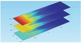
We've made a parametric extrusion. The different slices show the electric field on the pyramidal unit cell for the selected values of  $\theta$ .
