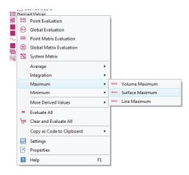
This allows us to evaluate the maximum of a chosen variable over a surface domain. In the Surface Maximum settings window, we'll choose Study 1/Parametric Solutions 1 for the data set. Set the selection to Domain 1 by clicking on the cross-section of the pulley shown in the Graphics window.
