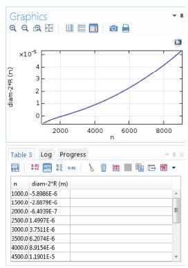
Results show the table and graph indicating how the deformation increases with higher rpms.
