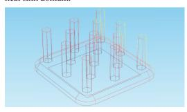
Line plots can also be used to show results at multiple locations in a model. Under the Coloring and Style tab in the settings for a line plot, the style can be set to lines or to tubes, with a manually-adjustable radius.
