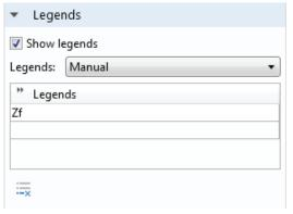
To change the location of the legend box, go to the main plot group node (1D Plot Group 1) and expand the Legend tab. The position can be set to top, middle, and bottom heights in the left, right, and middle sections of the grid.
