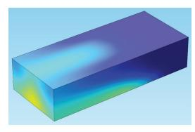
In the Surface settings window, we can change this under the Coloring and Style tab. Using the drop-down list, change the color table from Rainbow to ThermalLight.
