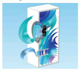
This model studies how the sensitivity of a loudspeaker driver is affected by its enclosure. The speaker driver is set in a vented enclosure and contains a magnet, voice coil, cone, and other hardware components. The simulated air domain is surrounded by a spherical perfectly matched layer (PML) that absorbs outgoing waves, minimizing reflections in order to model an infinite domain.
