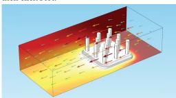
Now the arrow plot shows the velocity of the airflow as it changes. The *Color legend* check box under the Coloring and Style tab allows you to see a reference for the fastest and slowest flow regions (with red being the fastest, blue the slowest).
