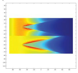
The second surface plotted right on top of the first one, causing our earlier results to vanish. We need to add a deformation so that we can see these results side by side.
