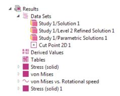
Three solutions have already been created. They are different result sets from the same study; Study 1/Level 2 Refined Solution 1 includes a step in the study that refines the mesh in certain areas of the model where greater accuracy is needed, while Study 1/Parametric Solutions 1 includes results from the parametric sweep performed in the study.
