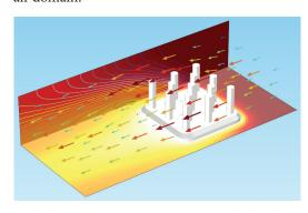
Instead of lines, we can also blend the contours so that the space between each level is filled in. Check out the options available in the Levels tab and the Coloring and Style tab in the Contour settings window:
