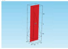
Go back to the Surface node in 2D Plot Group 3, make sure that the data set is set to Cut Plane 1, and click Plot. Now we have results:
