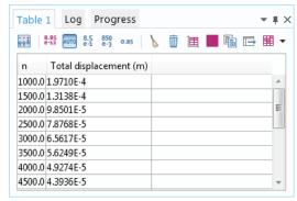
We can also add multiple variables to this table. Add the expression *solid.mises* (von Mises stress) by typing it in or clicking Replace Expression and choosing *Model* > *Component 1* > *Solid Mechanics* > *Stress* > *solid.mises* - *von Mises stress*. Change the units to *MPa* and click Evaluate again.
