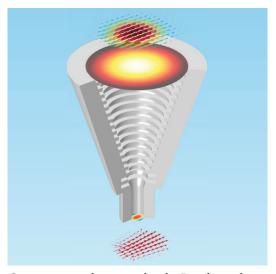
Create a new solution under the Results node, Study 1/Solution 1 (5). Add a selection that includes domains 3, 4, and 6 (the horn, feed, and aperture). Then right-click Data Sets and choose *Revolution 2D*. Choose Study 1/Solution 1 (5) as the data set and use a start angle of -90 degrees and a revolution angle of 225 degrees.
