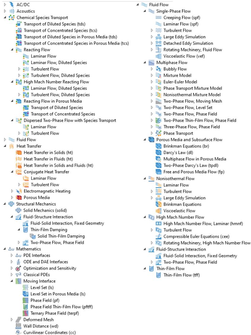
Figure 6: The physics interfaces for the CFD Module as shown in the Model Wizard (left: the full set of physics interfaces with the included physics interfaces in the Chemical Species Transport, Heat Transfer, Structural Mechanics, and Mathematics branches expanded; right: the fully expanded Fluid Flow branch).
