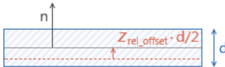
Figure 7-2: Meshed boundary indicated in red. The vector \mathbf{n} indicates the positive orientation of the boundary normal.
