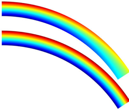
Figure 2-15: xx -components of the Cauchy stress tensor (top) and Second-Piola-Kirchhoff stress tensor (below) for an initially straight beam
