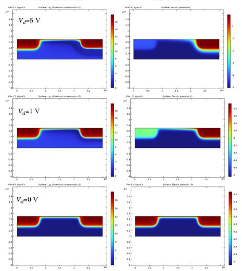
Figure 10: Electron concentration and electric potential distribution at Vd values of 0, 1 and 5 V. The pinch-off of the channel is apparent at 5  $\rm V$ .
