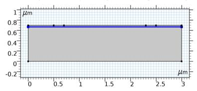
3 Click the Build All button to build the entire geometry. Use the Zoom Extents button at the top of the Graphics window to zoom to the full geometry if desired. Notice that the interior line is not shown in the finalized geometry, because it is defined as a Mesh Control Edge in the previous step and will only appear when we set up the mesh later.
