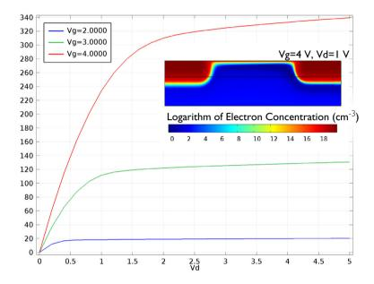
Figure 2: Stationary analysis of a MOSFET. The plot shows the drain current plotted against the drain voltage  $(V_d)$  for a range of different values of the gate voltage  $(V_d)$ . The inset shows the logarithm of the electron concentration (in units of cm<sup>-3</sup>) for a gate voltage of 4 V and for a drain voltage of 1 V. The channel is clearly visible.
