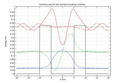
The Schrödinger-Poisson Equation interface adds the Electrostatics physics to take into account the effects of the charge density of the carriers. The following graph shows the self-consistent result of electrons confined in a quantum wire.
