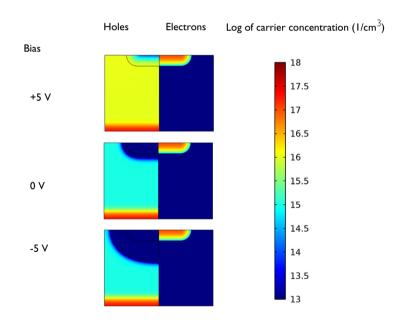
Figure 1: Electron and hole concentrations in a p-n junction diode connected to a series resistor under different bias conditions. This plot shows clearly the changing geometry and extent of the depletion region under reverse bias.
