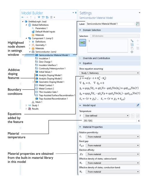
Figure 5: The Model Builder (to the left), and the Settings window for Semiconductor Material Model I for the selected feature node (to the right). The Equation section in the Settings window shows the model equations.
