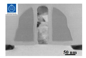
Figure 8: Cross-section TEM (transmission electron microscopy) image of a 50 nm gate length MOSFET fabricated at KTH Electrum laboratory by P.E. Hellström and coworkers within the ERC advanced grant OSIRIS research project headed by Prof. M. Östling.
