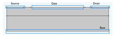
Figure 9: Model geometry showing the external connections.
