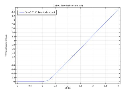
From the plot it is clear that the threshold voltage,  $V_T$ , of the transistor is approximately 1.2 V. It is possible to compare this value with the theoretical value given by (S. M. Sze and K. K. Ng, *Physics of Semiconductor Devices*, Wiley, Hoboken, New Jersey, pp. 305–306, 2007):
