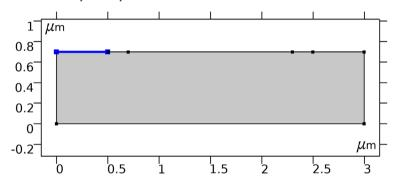
**Note:** The Metal Contact feature in COMSOL Multiphysics is a so called Terminal boundary condition. By default a fixed potential of 0 V is applied, which is appropriate in this instance, since the source is grounded. The terminal can also be set up to specify an input current, input power, or to connect to a voltage or current source from an external circuit.
