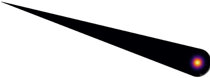
*Release of a Gaussian beam from a point. The ray power is a Gaussian function of the release angle. This type of power distribution is appropriate when the geometry is much larger than the Rayleigh range.*
