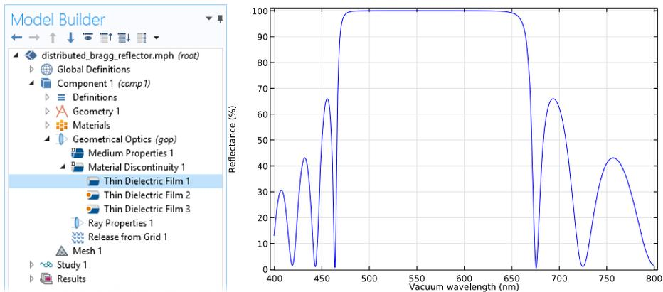
*Distributed Bragg Reflector (DBR): Several thin dielectric films can be added to the same boundary, and these layers can be made periodic with a large number of unit cells. Here the reflectance of a DBR with 21 dielectric layers is plotted as a function of wavelength.*
