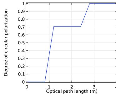
*Linearly polarized light is internally reflected twice in a Fresnel rhomb (left). As a result, the ray's polarization ellipse shifts from linear, to elliptical, to circular. This can also be shown by plotting the degree of circular polarization plotted as a function of optical path length (right).*
