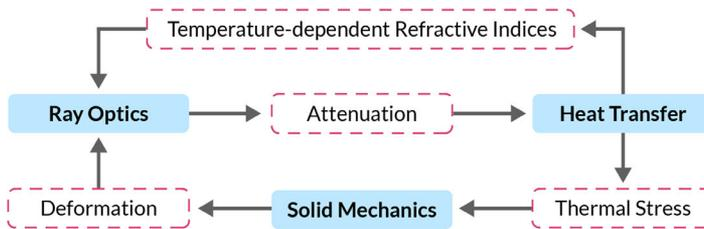
*Bidirectional coupling between ray optics and heat transfer, including thermal stress.*
