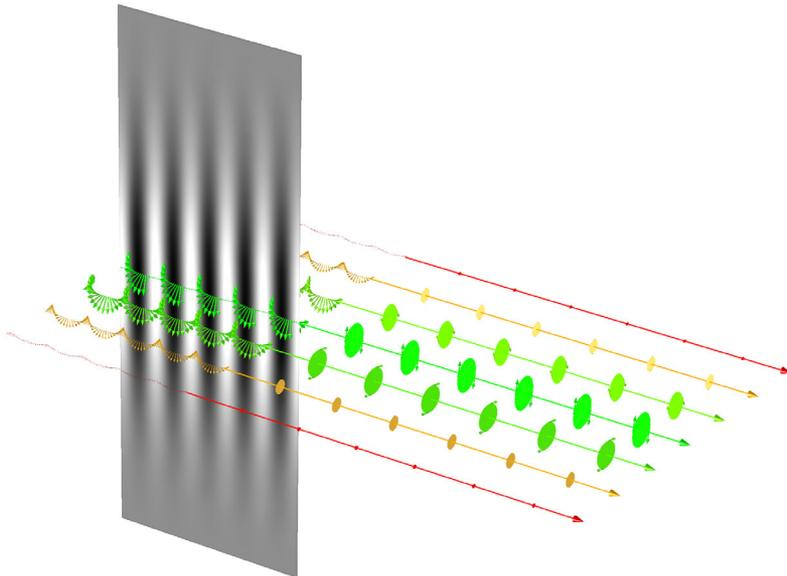
The propagation of a Gaussian beam is modeled using the Electromagnetic Waves, Beam Envelopes interface. Then rays are released from the adjacent surface. The rays are assigned their initial intensity and polarization based on the tangential electric field. Polarization ellipses are drawn along the rays.
