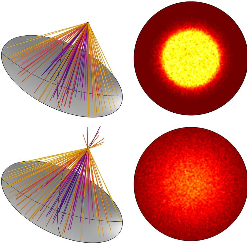
*Rays released from an illuminated solar reflector and resulting concentration ratios in the focal plane. The top row is the ideal case. The bottom row includes surface roughness and solar limb darkening effects.*
