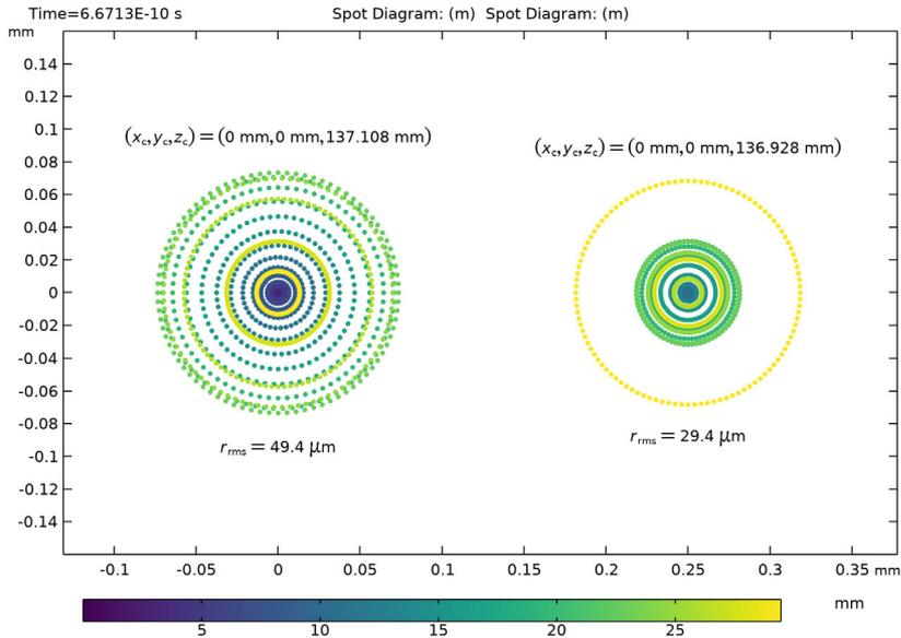
The double Gauss lens spot diagram. On the left is the spot on the nominal image surface. The spot on the right is located at the "best focus" image plane that has been computed automatically.
