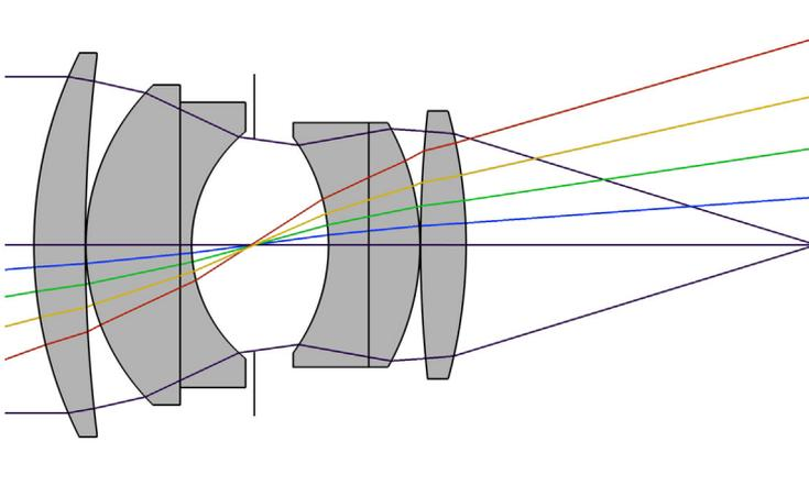
*Overview of a double Gauss lens. In this view the marginal rays of an on-axis trace are shown, together with the chief ray of 4 additional fields.*
